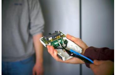
The already existing handheld E-band radar demonstrator is to be scaled to D-band. The frontend comprises a transmitter and receiver. On-PCB antennas are situated on the right-hand side of the PCB.
