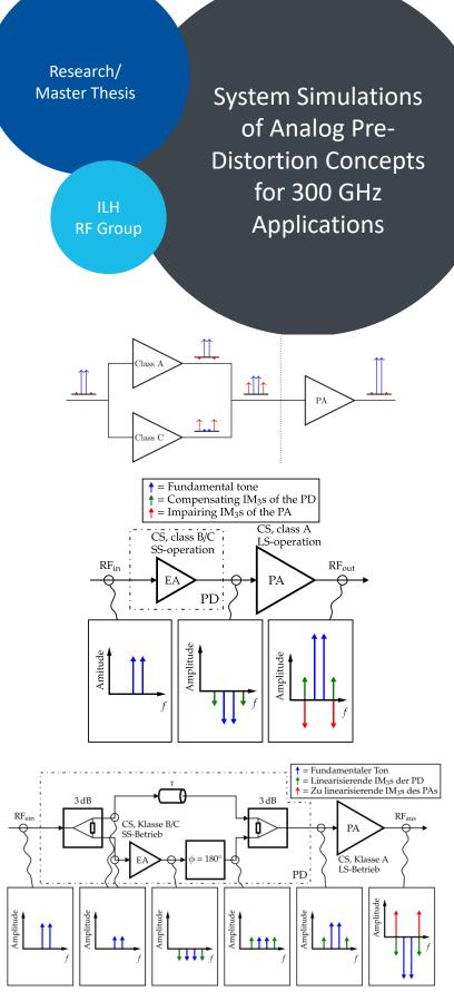
Three analog pre-distortion concepts, subject to investigation. All concepts try to enhance the PAs linearity by injecting compensating signal components.
