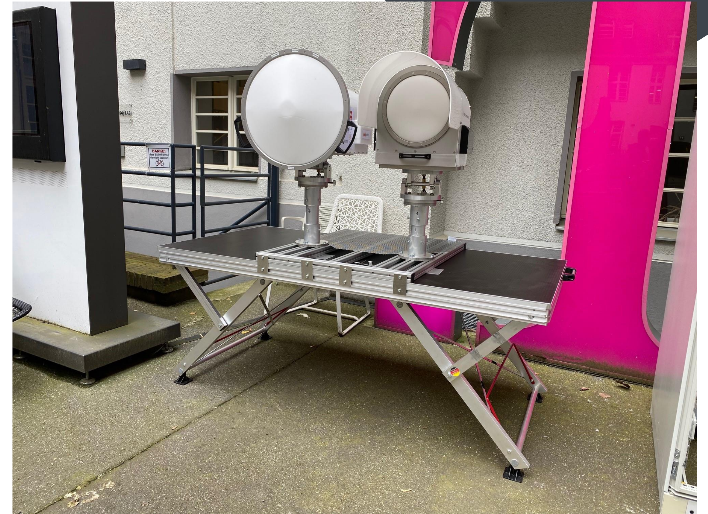
Highly directive H-band Cassegrain antenna systems
