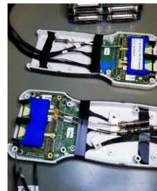
Self-mixing radar demonstrator front-end (E-band) and scheme with independent Tx and Rx
