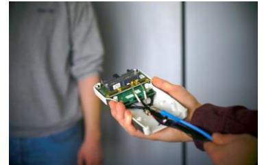
Already existing handheld E-band radar demonstrator to be scaled to D-band. The frontend comprises a transmitter and receiver. On-PCB antennas situated on the right-hand-side of the PCB.
