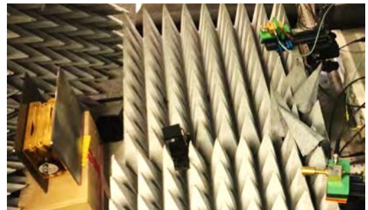
Hybrid measurement setup of a stepped frequency continuous wave radar of a preceding work
