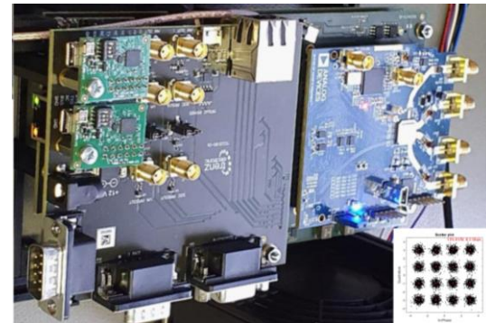
[EIVE Digital Baseband (flight HW), in the function of Arbitrary Waveform Generator (AWG) based on multiMIND Platform]
